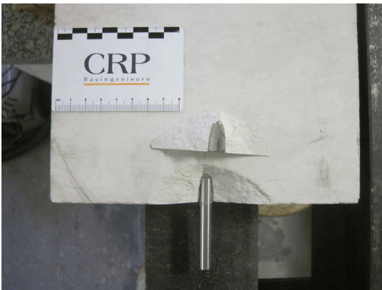
Photo 2 Pin of 8 mm, manner of breaking during testing
