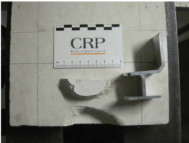
Photo 4 Clip B, manner of breaking during testing
