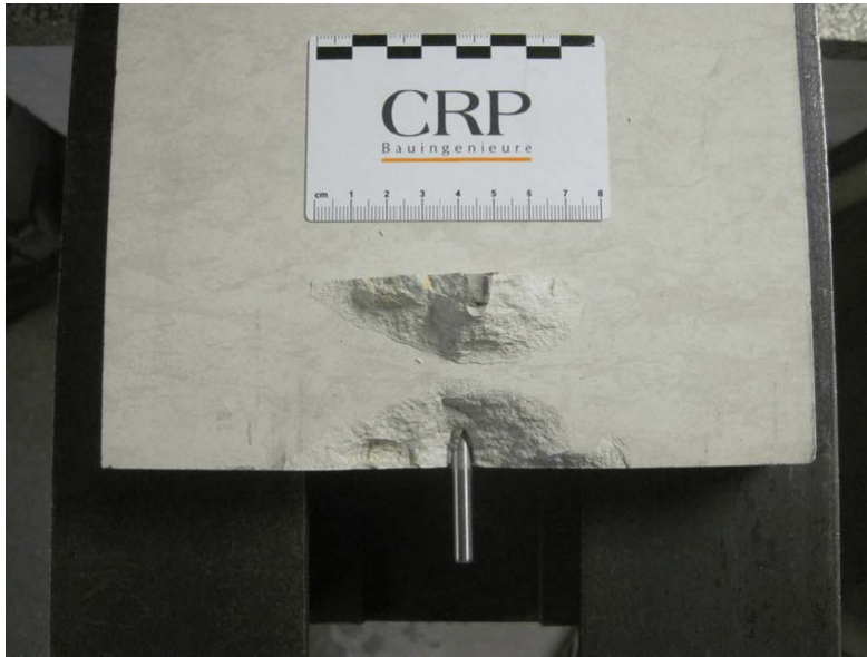
Photo 1 Pin of 6 mm, manner of breaking during testing
