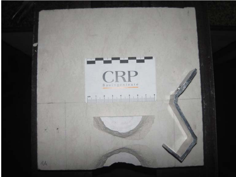
Photo 3 Clip A, manner of breaking during testing
